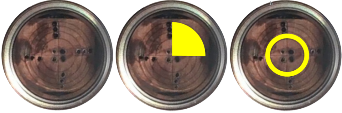
Figure 5: Photograph of the voltage detector in the Gabor lens. The detector is composed of 16 segments, connected in groups of four, either in segments, left, or in concentric circles, right.
