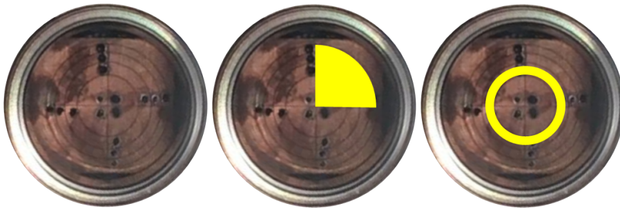
Figure 10: A photograph of the 16-segment detector in different arrangements: sector (middle), concentric circle (right)
