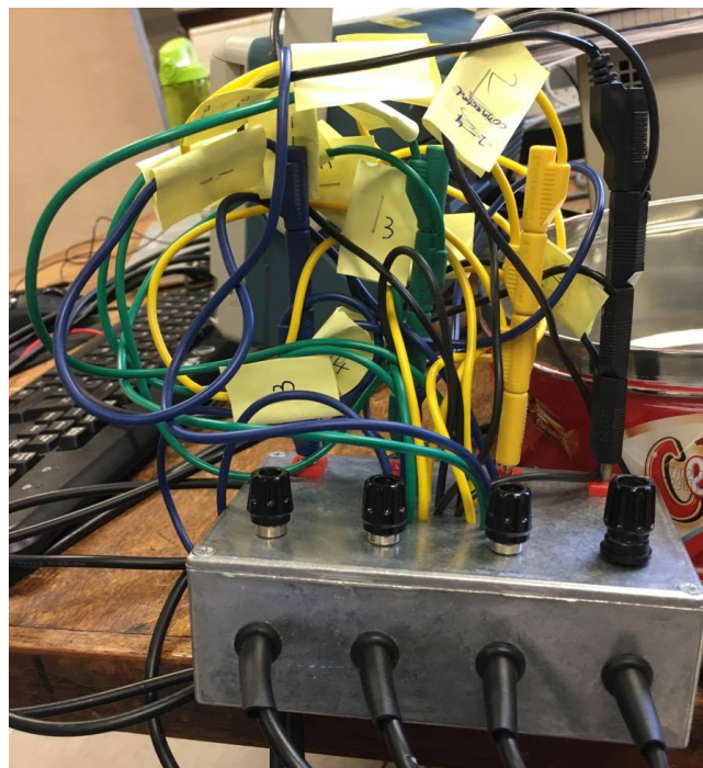
Figure 11: A photograph of the 16-segment detector fed into the junction box in the sector arrangement, each segment has a colour and a number labeled on the wire
